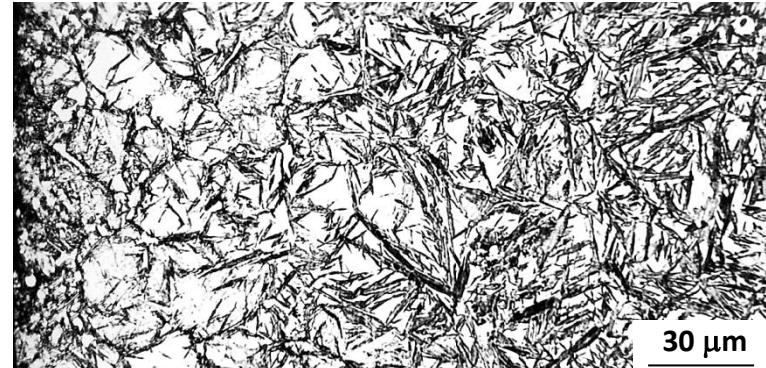
Retained austenite, net of secondary cementite
